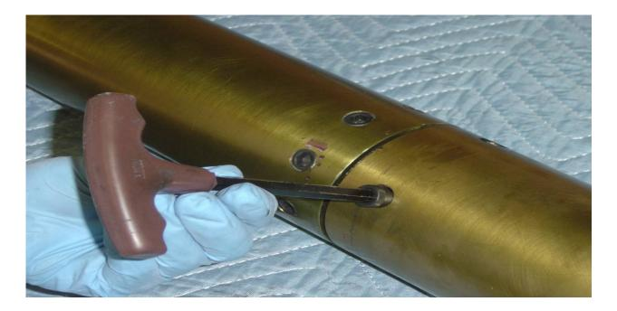
**Step 7:** Grease the Injector Baffle O-rings and slide the nitrous tank section of the motor onto the combustion chamber and insert the retention bolts. The bolts will require a 5/16 inch hex head wrench.
