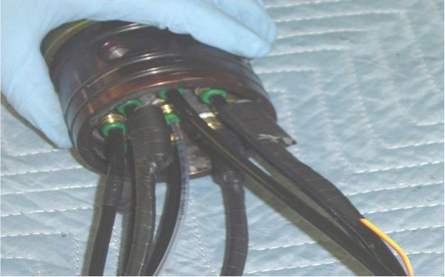
**Step 5:** Insert the Fill lines w/ Pyrodex Pellets attached into the injector baffle on opposite sides. Ensure that the nylon lines go all the way into the press locks and go past the O-Ring Seal. You will feel it go past the O-ring and seat at the bottom of the fitting. You will now insert the clear vent line into the center fitting, and the short crossover line/lines into the last fittings. Ensure that all the lines are secure in the fittings prior to moving on.
