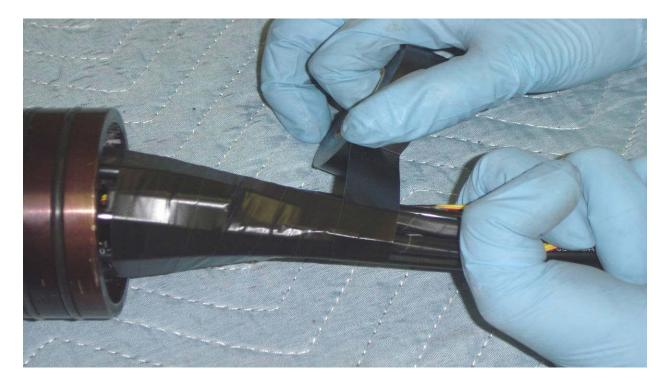
**Step 6:** Using your roll of electrical tape, start taping around all nylon lines. This will slightly pull the lines towards the center of the motor, and ensure the heat of the Pyrodex Pellets at ignition is kept near the lines to ensure a positive ignition. You will only need a single layer of tape over the line set to hold them together.
