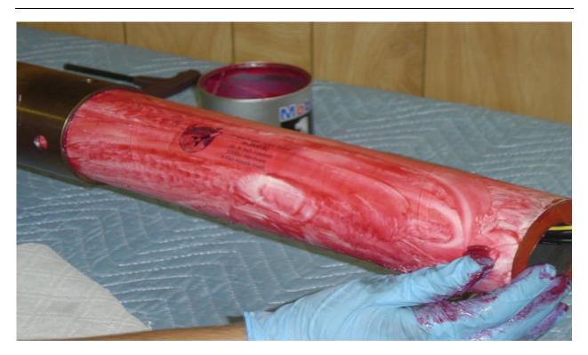
**Step 8:** Grease the included fuel grain with a synthetic type grease (Mobile 1 or similar) and slide the fuel grain into the combustion chamber. Ensure that the fill lines, vent line and igniter wires are all drawn through the core of the grain. A thin coating of grease is all that is required.
