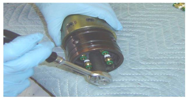
**Step 3:** Insert Press Lock Fittings into the Injector Face. A 1/8 Inch Fitting will always go in the center port. The Fittings should be tightened <sup>1</sup>/<sub>2</sub> turn past tight. If only 4 Injectors are used (Slow and Medium Motors) the Injectors should alternate radically with a steel plug. (4 Steel Plugs will be included with the necessary reloads)
