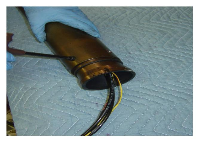
**Step 9:** Grease the Nozzle O-rings and slide the nozzle into the combustion chamber. If you will be using a retaining ring on the nozzle, be sure to put this onto the nozzle prior to bolting it into the combustion chamber.
