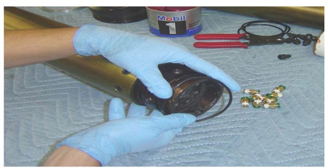
**Step 2:** Begin by installing all O-Rings onto Nozzle and Injector Baffle. All O-rings are Dash Number 236. O-Rings should be free from any cracks, burns or damage.
