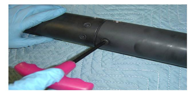
**Step 7:** Grease the Injector Baffle O-rings and slide the nitrous tank section of the motor onto the combustion chamber and insert the retention bolts. The bolts will require a <sup>1</sup>/<sub>4</sub> inch hex head wrench.
