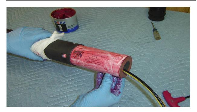
**Step 8:** Grease the included fuel grain with a synthetic type grease (Mobile 1 or similar) and slide the fuel grain into the combustion chamber. Ensure that the fill lines, vent line and igniter wires are all drawn through the core of the grain. A thin coating of grease is all that is required.
