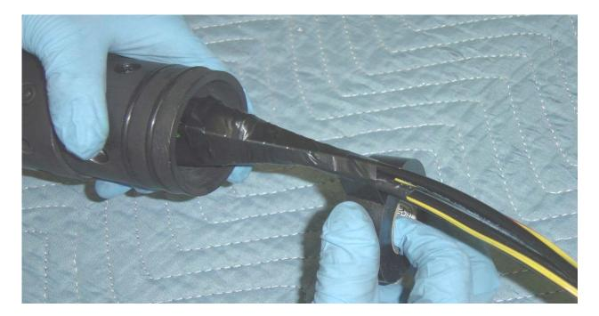
**Step 6:** Using your roll of electrical tape, start taping around all 5 nylon lines. This will slightly pull the lines towards the center of the motor, and ensure the heat of the Pyrodex Pellets at ignition is kept near the lines to ensure a positive ignition. You will only need a single layer of tape over the line set to hold them together.
