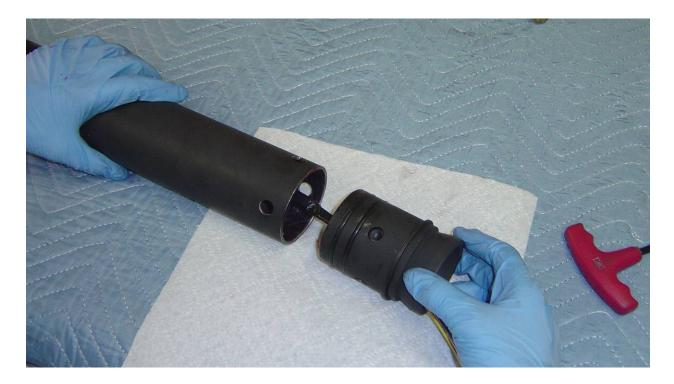
**Step 9:** Grease the Nozzle O-rings and slide the nozzle into the combustion chamber. If you will be using a retaining ring on the nozzle, be sure to put this onto the nozzle prior to bolting it into the combustion chamber.
