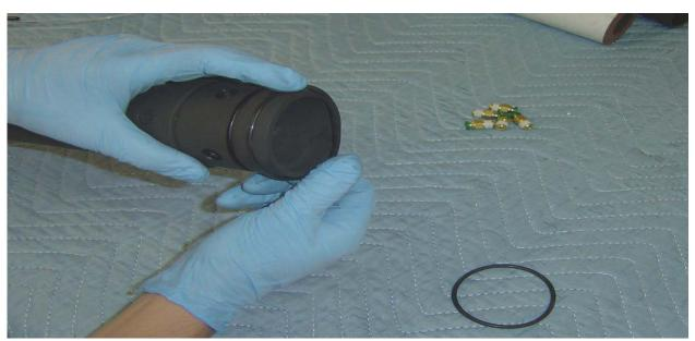
**Step 2:** Begin by installing all O-Rings onto Nozzle and Injector Baffle. All O-rings are Dash Number 230. O-Rings should be free from any cracks, burns or damage.
