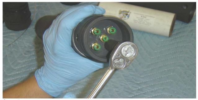
**Step 3:** Insert Press Lock Fittings into the Injector Face. A 1/8 Inch Fitting will always go in the center port. 1/8 inch Fittings are used for Slow Motors, 3/16 for Medium Motors and 1/4 Inch for Fast Motors. The Fittings should be tightened  $\frac{1}{2}$  turn past tight.
