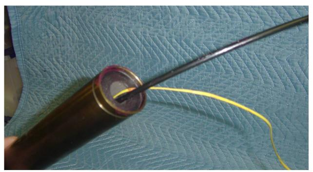
**Step 10:** Slide the Fuel grain into the motor case by pushing it down, which will also push the injector assembly into position as well. Wipe any excess grease off of the outside of the motor case.
