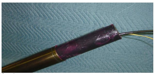
**Step 9:** Find the included Fuel Grain which came with the reload package. Grease the outside of this grain with a non-petroleum based grease. We recommend Mobile 1 Synthetic Grease. Completely cover the grain with grease before sliding the grain onto the fill line and igniter wire.
