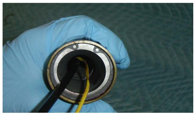
**Step 12:** Be sure that the nozzle and nozzle washer are pressed slightly below (approx. 1/16<sup>th</sup> of an inch) the snap ring groove. Find the second snap ring, and insert the snap ring into the groove to complete motor assembly.
