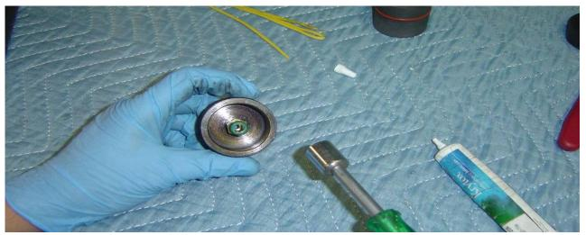
**Step 5:** Install Parker Press-Lock Fitting into the Floating Injector. (The Floating Injector is denoted by an "I" Stamped on the top face) This should be done with a deep wall socket set. Make sure the injector is tightened to ½ turn past snug. To verify injector speeds and Igniter requirements please view the attached chart.
