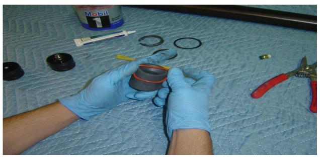
**Step 2:** Begin by installing all O-Rings onto Nozzle, Injector Baffle, and Bulkhead. All O-rings are Dash Number 223. O-Rings should be free from any cracks, burns or damage.
