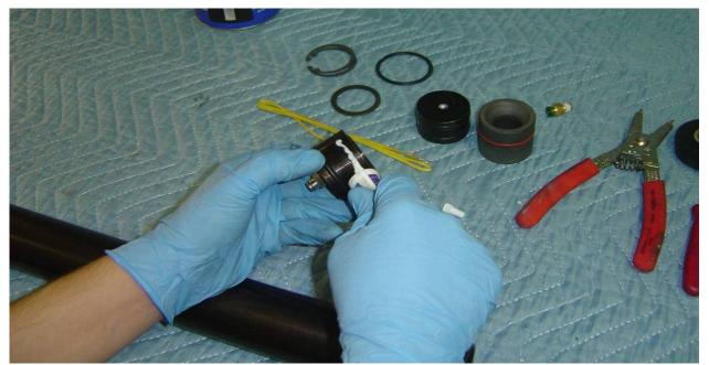
**Step 3:** Use Krytox<sup>TM</sup> grease on top Bulkhead O-rings. Smear Krytox<sup>TM</sup> over the entire outer cylindrical surface of the Bulkhead. This allows for an easy fit into the motor case. Krytox grease is available from Contrail Rockets and our Dealers.
