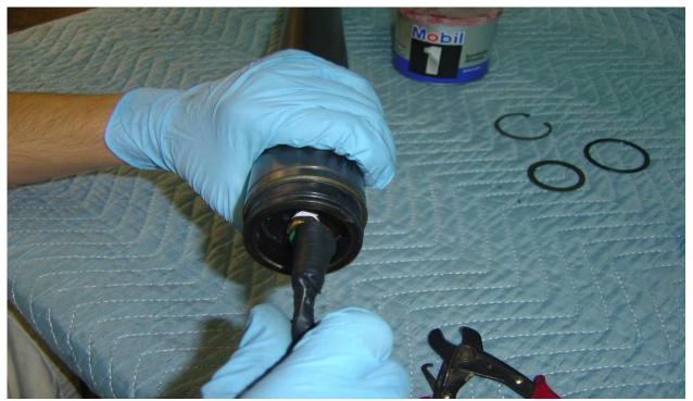
**Step 8:** Now that the Injector and Igniter assembly is put together, you will be greasing the Injector Assemble with Krytox<sup>TM</sup> Grease just as you did with the top bulkhead. Once the Injector is greased you will slide the assembly into the motor tube. Be sure to not slide the injector up to far, as you will use the grain to push the injector up the rest of the way into the case.
