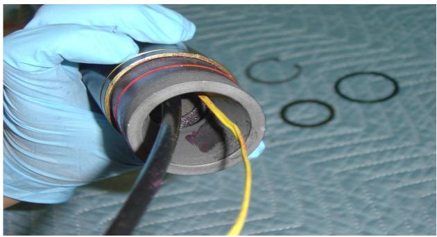
**Step 11:** Find the graphite nozzle with O-ring and give a light coat of synthetic grease. You then want to slide the graphite nozzle into the motor case. Following the insertion of the nozzle into the motor case you will then place the nozzle washer onto the face of the nozzle.
