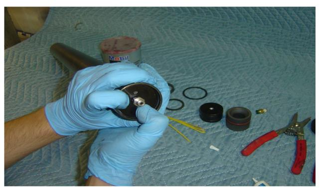
**Step 4:** Slide top bulkhead into the top side of the motor case. (The top of the motor case does not have an external groove cut into it for a thrust washer). Once the bulkhead is pushed just below the snap ring groove, install the snap ring using snap ring pliers.
