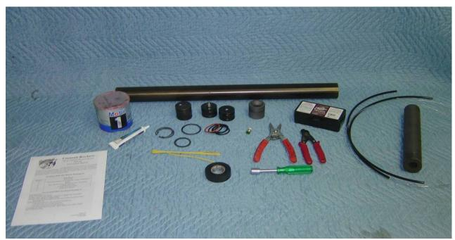
**Step 1:** Ensure that your motor hardware is clean and free from grease, oils, dirt and debris. Wipe the motor components with soap and water, to cut any residual grease from previous firings. Make sure you have all required tools and parts for motor assembly.
