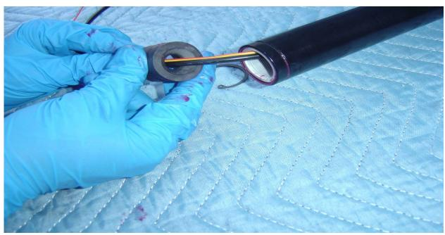
**Step 13:** Find the graphite nozzle with O-ring and give a light coat of synthetic grease. You then want to slide the graphite nozzle into the motor case. Following the insertion of the nozzle into the motor case you will then place the nozzle washer onto the face of the nozzle.
