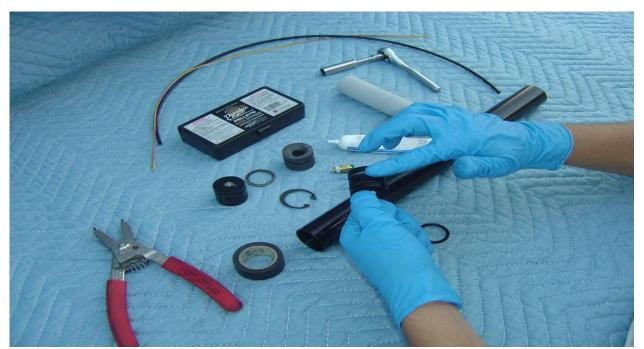
**Step 3:** Use Krytox<sup>TM</sup> grease on top Bulkhead O-rings. Smear Krytox<sup>TM</sup> over the entire outer cylindrical surface of the Bulkhead. This allows for an easy fit into the motor case. Krytox grease is available from Contrail Rockets and our Dealers.
