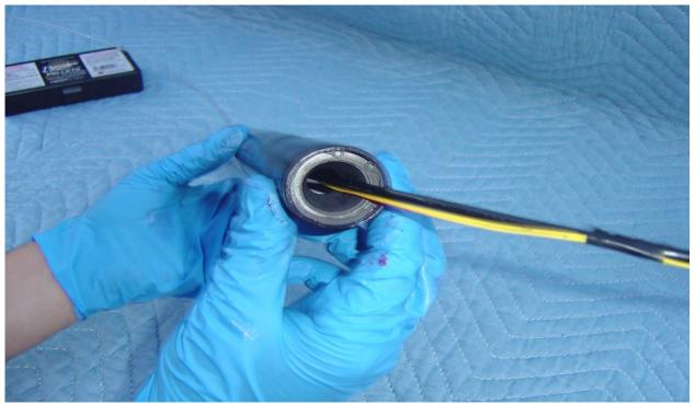
**Step 14:** Be sure that the nozzle and nozzle washer are pressed slightly below (approx. 1/16<sup>th</sup> of an inch) the snap ring groove. Find the second snap ring, and insert the snap ring into the groove to complete motor assembly.
