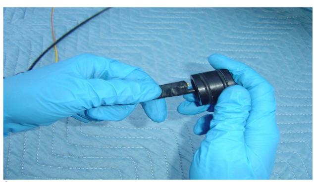
**Step 9:** After aligning the igniter into position, use electrical tape to tape the igniter to the fill line. 2 wraps of electrical tape over the entire igniter grain is recommended. This holds the heat of the Black Powder Pellets close to the Nylon Line.
