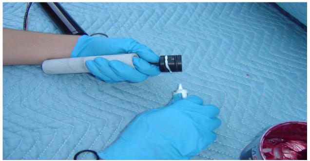
**Step 10:** Now that the Injector and Igniter assembly is put together, you will be greasing the Injector Assemble with Krytox<sup>TM</sup> Grease just as you did with the top bulkhead. Once the Injector is greased you will slide the assembly into the motor tube. Be sure to not slide the injector up to far, as you will use the grain to push the injector up the rest of the way into the case.
