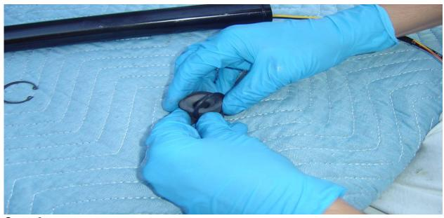
**Step 2:** Begin by installing all O-Rings onto Nozzle, Injector Baffle, and Bulkhead. All O-rings are Dash Number 215. O-Rings should be free from any cracks, burns or damage.
