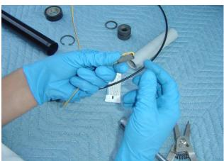
**Step 7:** Refer to the Igniter/Injector Chart to find out which size and number of Pyrodex Pellets is recommended for ignition. Verify that you have the correct size and number of Pyrodex Pellets for your reload and then slide the igniter wire through the center hole of the pellet. Bend the resistor to the side of the powder pellet as shown.
