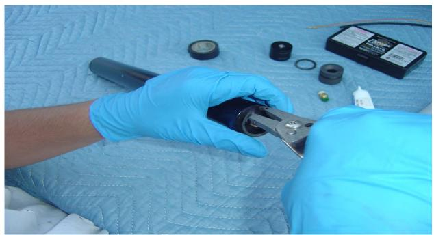
**Step 4:** Slide top bulkhead into the top side of the motor case. (The top of the motor case does not have an external groove cut into it for a thrust washer). Once the bulkhead is pushed just below the snap ring groove, install the snap ring using snap ring pliers.
