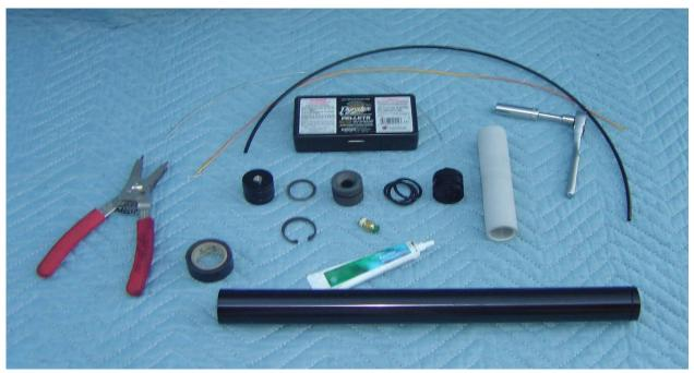
**Step 1:** Ensure that your motor hardware is clean and free from grease, oils, dirt and debris. Wipe the motor components with soap and water, to cut any residual grease from previous firings. Make sure you have all required tools and parts for motor assembly.
