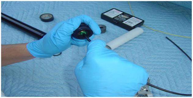
**Step 6:** Find the included Nylon Fill Line, and make sure the nylon line is cut square. If it is not, use a set of cutters to square off the end of the lines. Once the line is cut square, push the line into the Press Lock Fitting. Be sure that you feel the fitting go past an O-Ring seal and seat snugly onto the bottom of the fitting. Once Seated give a slight pull to ensure the fitting is locked in, and the fittings "Teeth" grab onto the line.
