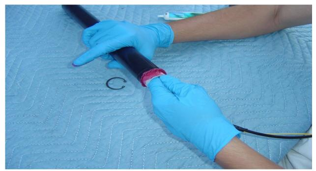
**Step 12:** Slide the Fuel grain into the motor case by pushing it down, which will also push the injector assembly into position as well. Wipe any excess grease off of the outside of the motor case.
