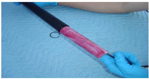
**Step 11:** Find the included Fuel Grain which came with the reload package. Grease the outside of this grain with a non-petroleum based grease. We recommend Mobile 1 Synthetic Grease. Completely cover the grain with grease before sliding the grain onto the fill line and igniter wire.
