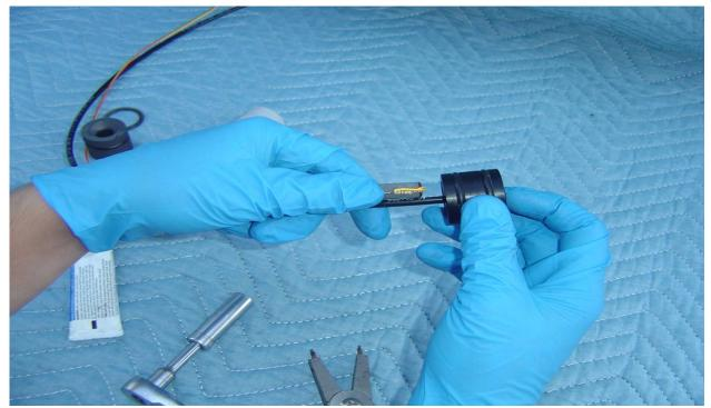
**Step 8:** Place the Igniter assembly next to the top of the Injector Face. Put the Resistor approximately 90 Degrees away from the fill tube. (Refer to Picture).
